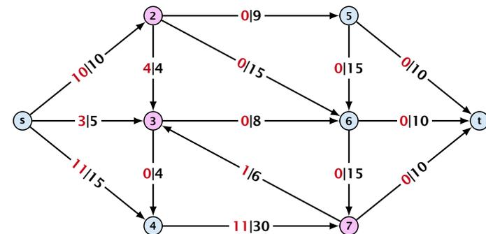
A node that has  $\sum_{e \in \text{out}(v)} f(e) < \sum_{e \in \text{into}(v)} f(e)$  is called an **active node**.
