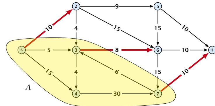
The capacity of the cut is  $\text{cap}(A, V \setminus A) = 28$ .
