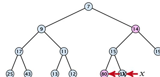
Note that an exchange can either be done by moving the data or by changing pointers. The latter method leads to an addressable priority queue.
