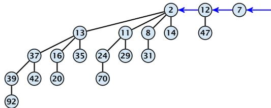
In a binomial heap the keys are arranged in a collection of binomial trees.
