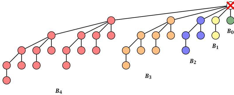
Deleting the root of  $B_5$  leaves sub-trees  $B_4$ ,  $B_3$ ,  $B_2$ ,  $B_1$ , and  $B_0$ .
