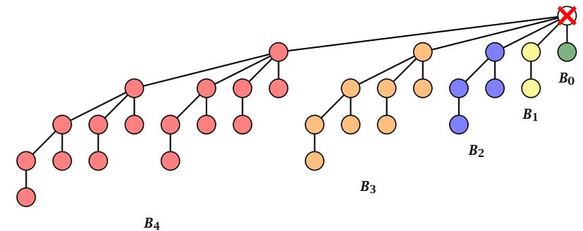
Deleting the root of  $B_5$  leaves sub-trees  $B_4, B_3, B_2,$  and  $B_1$ .
