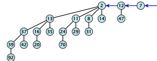
In a binomial heap the keys are arranged in a collection of binomial trees.
