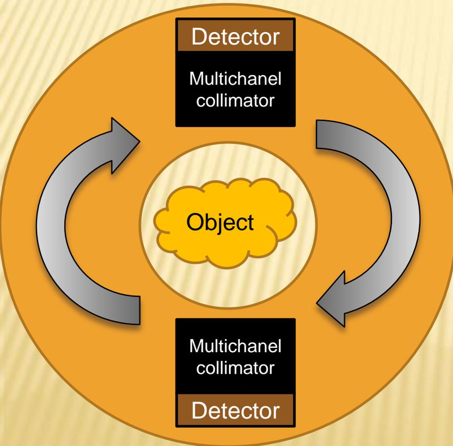
Diagnostic scheme with usage coded aperture
