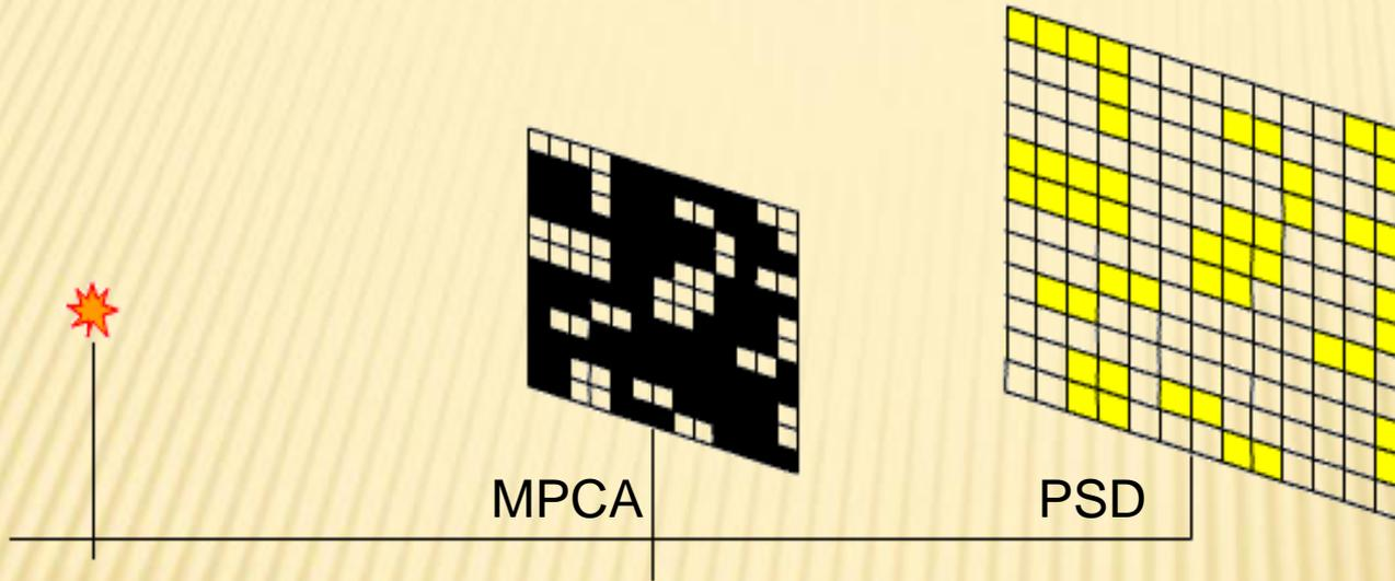
The shadow on the detector is a copy of the coded aperture. Decoding is required
