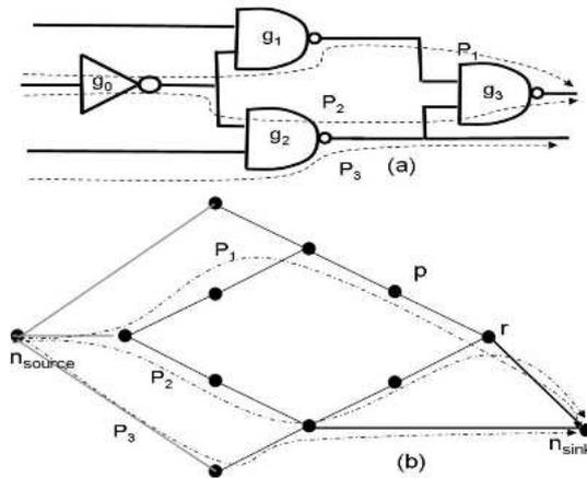
Figure 8: Combinational circuit and its corresponding DAG[1]
