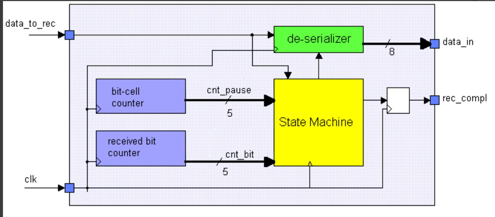
Receiver is used for receiving data from 1 bit input and to transform this data to 8 bit output.
