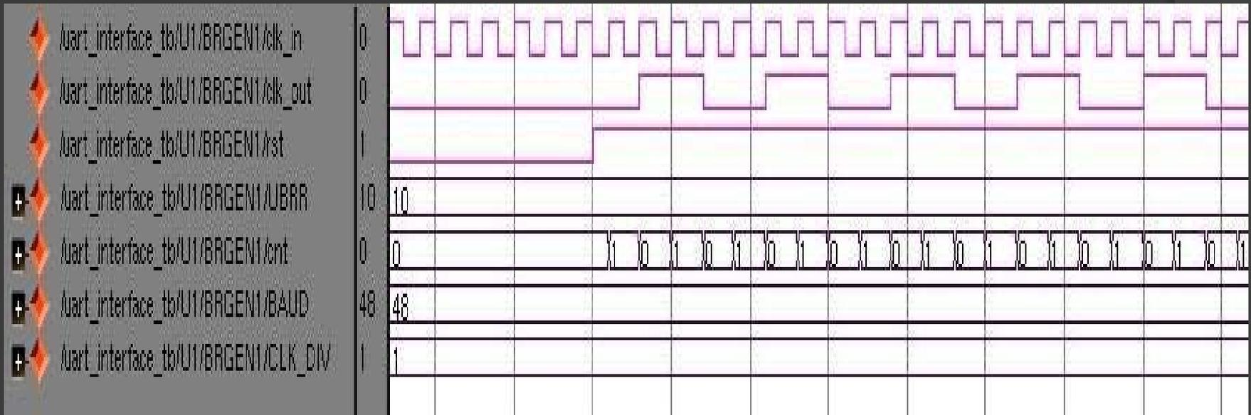
To make baud rate generator operate we need to activate it. This picture shows activation process. Low level on RST input starts UART. After activation low level on RST resets UART.
