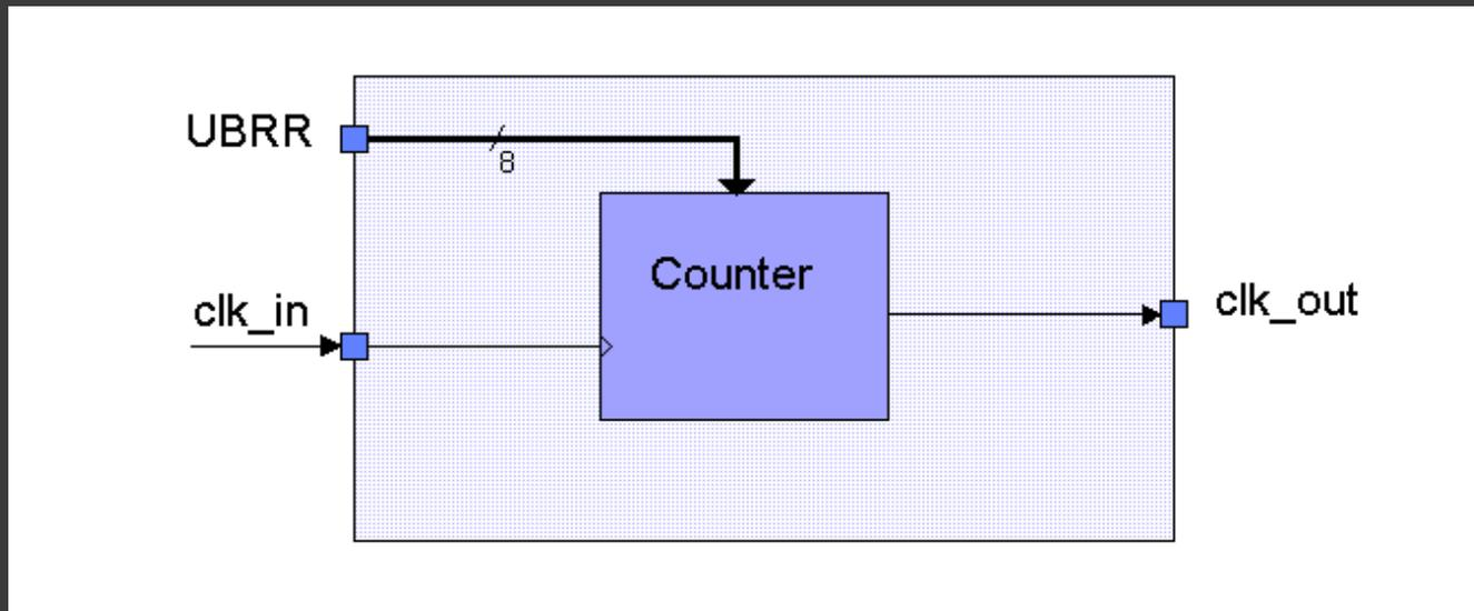
Baud rate generator is used for setting internal clock frequency and for changing transfer rate of UART.
