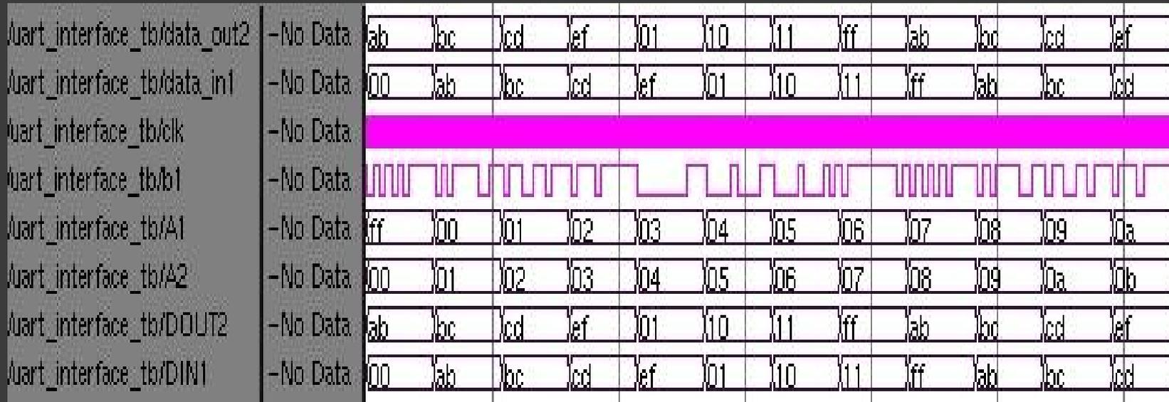
In this time 2 UART was connected to each other. First UART was transmitting data from 8x256 memory, and second UART was receiving incoming data and stored it in its empty memory.
