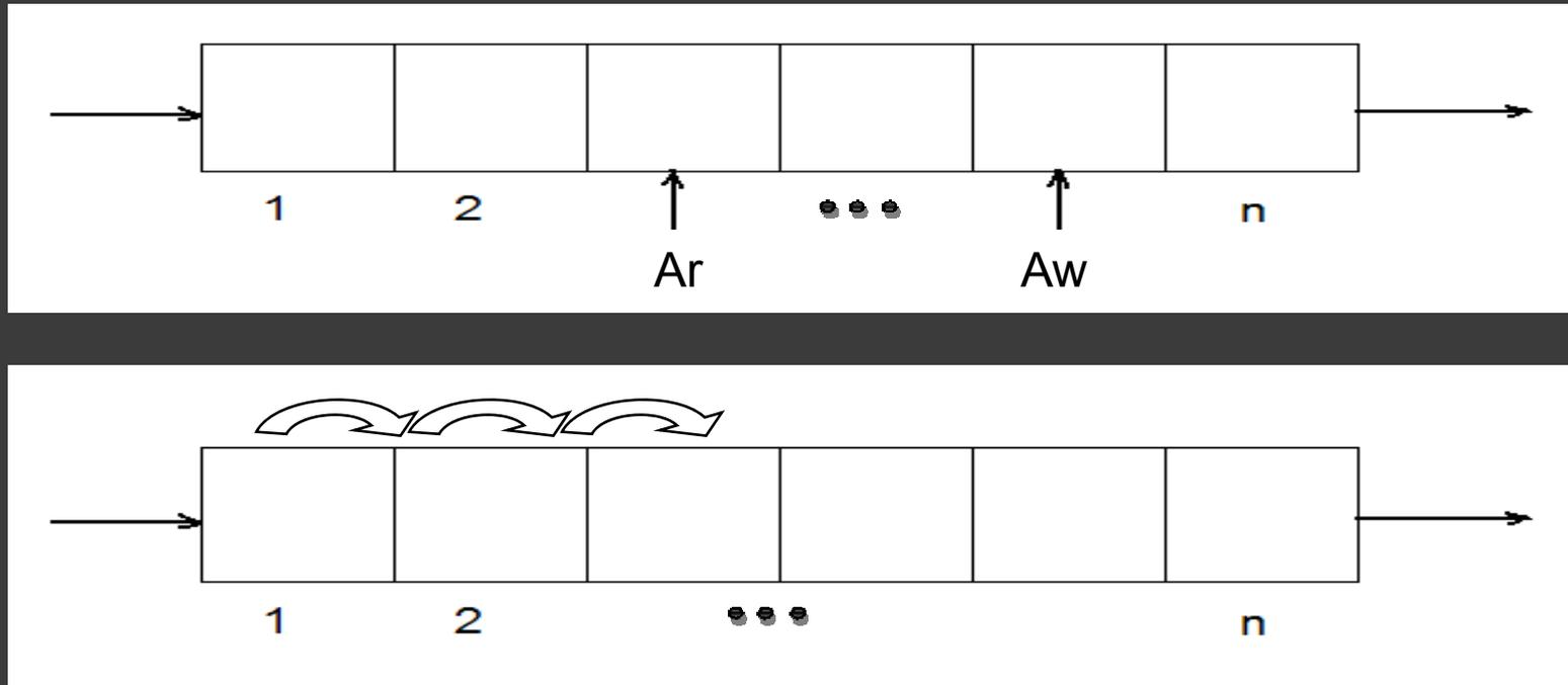
Incoming data is always stored in first cell of FIFO. After data is stored, shifting of data is performed. Because of this shifting, first inputted data would be always first to out.
