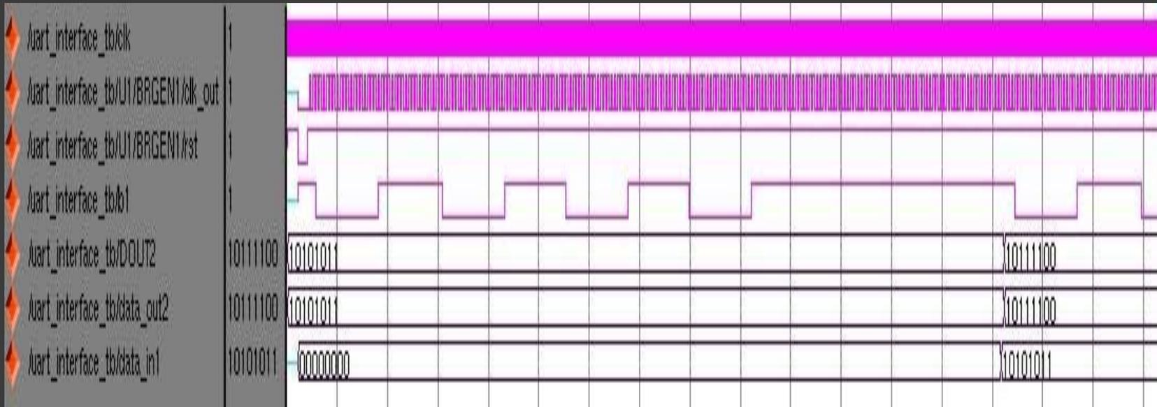
This figure shows transmitting 1 byte (10101011) with UART
