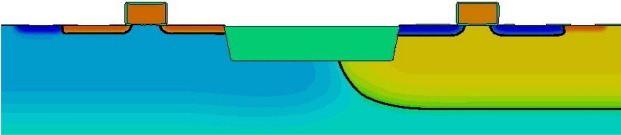
The modeling was performed using SDevices tool from TCAD Synopsys CAD package. We have researched effects in substrate during CMOS-gate switching. There is input and output signals and current through substrate.
