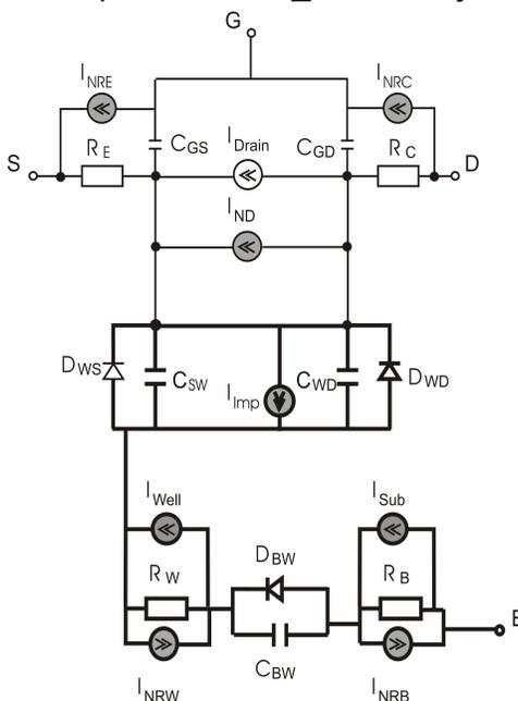
P-MOS transistor interacts with substrate similarly as n-MOS. As well p\_mos has current injection sources and sources that modeling p-mos interaction with substrate.
