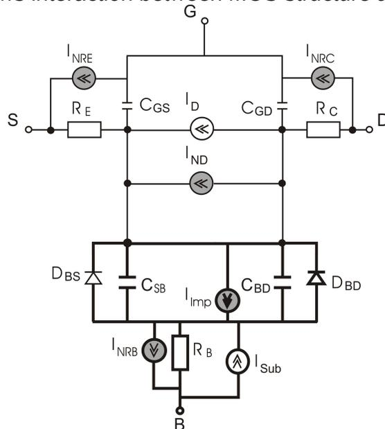
N-MOS transistor interacts directly with substrate through source-bulk and drain-bulk capacitances. On this equivalent circuits elements  $C_{db}$  and  $C_{sb}$  are modelling capacitances of the source-bulk and drain-bulk junctions. Dark sources are modeling noise sources of the diffusion regions. But more interested to see on the 2 elements that added in to equivalent circuits. This is:
