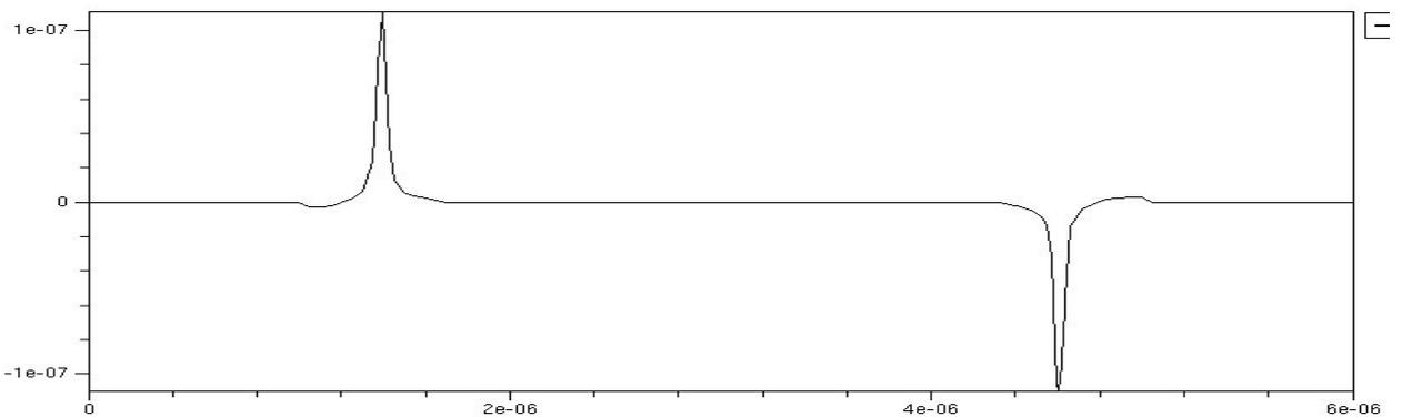
As was expected, we see current injection during switch process and fluctuation in current through substrate contact.
