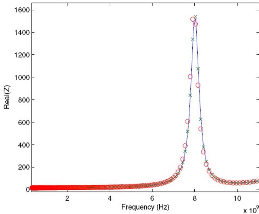
Fig.2 Real part of the impedance for the 3\*3 power grid. The original model denoted by solid line is unstable with order  $N=1566$ . Galerkin projection returns an unstable reduced model denoted by crosses. The core algorithm gives a stable reduced model denoted by circles
