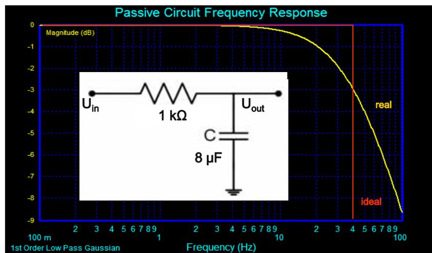
$$\text{Impedance of capacitor: } Z = 1/(\omega C) \rightarrow f_{co} = (RC)^{-1}$$
