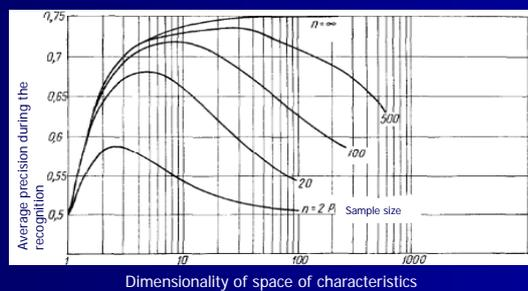
Fig. 4. Dependence of classification precision from dimensionality of space of characteristics
