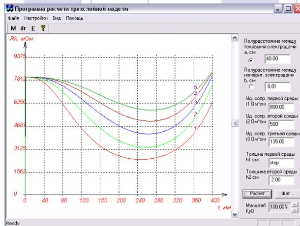
**Apparent resistivity vs. half interval between current electrodes**
