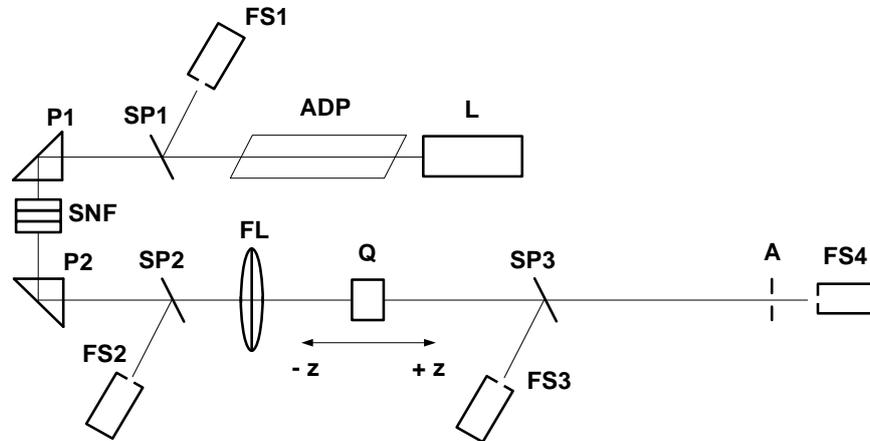
L - laser; ADP - nonlinear crystals - for the second harmonic generation ( $\lambda = 532 \text{ nm}$ ); FS - sensors; SP - semi-transparent plate; P - prisms; SNF - a set of neutral filters; FL - focusing lens; Q - cuvette; A - aperture
