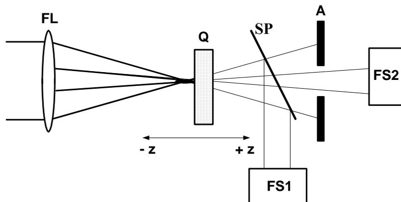
L - focusing lens; Q - cuvette; FS1, 2 - sensors; SP - semi-transparent plate; A - aperture
