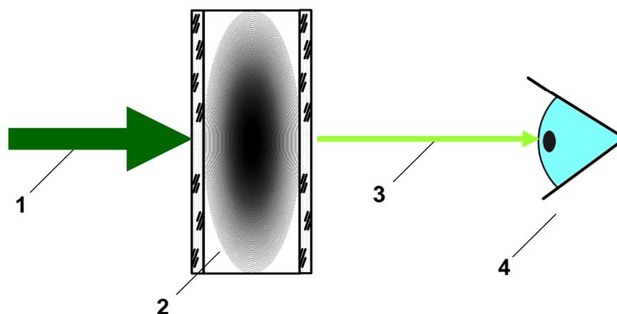
1 - high-intensity incident radiation, 2 - laser limiter, 3 - low-intensity output radiation, 4 – human eyes or sensitive elements of optical systems
