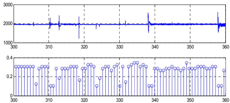
Receiving signal by radar and max frequency during troubled sleeping
