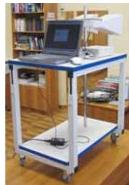
The bio-radar design has 16 operating frequencies in range of 3.6-4.0 GHz. The radar can measure the distance to a person under investigation and has improved abilities to filter noise and background reflections.
