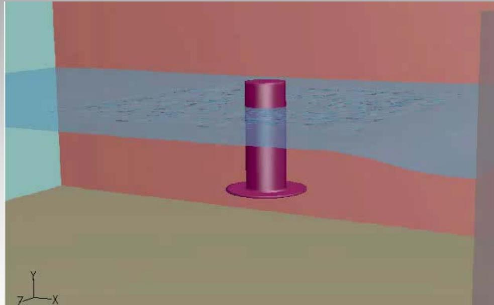
Simplified model of oil platform under wave load
