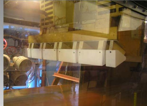
Scale (1:60) model of gate and ship passing channel
