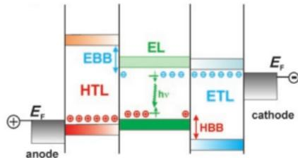
Hole and electron transfer layers to decrease the injection barriers
