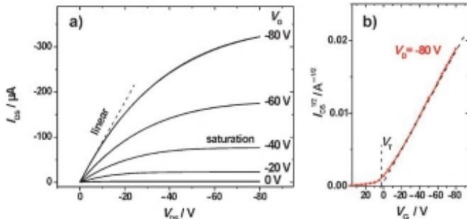
**Figure 14.** Examples of a)  $I_{DS}$ - $V_{DS}$  output characteristics and b)  $I_{DS}$ - $V_G$  characteristics of a prototypical OTFT comprising a  $\text{SiO}_2$ -hexamethyldisilazane (HMDS) gate insulator, Au top contacts, and P3HT as organic semiconductor. The hole mobility extracted from (b) was  $\approx 10^{-2} \text{ cm}^2 \text{ Vs}^{-1}$ . Device data kindly provided by D. Neher and P. Pingel (Universität Potsdam).
