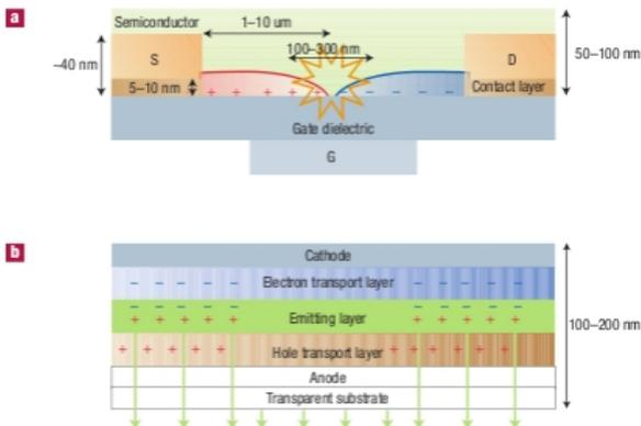
Useful for example in active matrix displays. No separate OLEDs and OTFTs needed → thinner and less complicated arrangement
