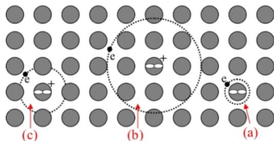
**(a) Frenkel exciton:** correlated  $e^-h^+$  pair that is located on the same molecule and moves as a unit through the crystal lattice.
