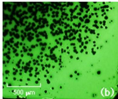
Dark spots on a ITO/ $\alpha$ -NPD/Alq<sub>3</sub>/Al OLED from: Kim et al.
