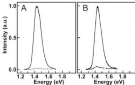
A) Excitation and B) emission spectra from InP nanowire (15nm diameter)
