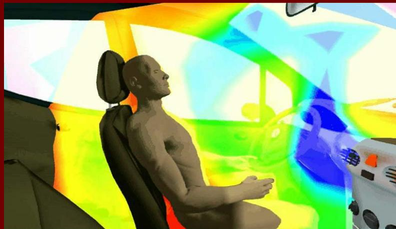
Color map of temperature spreading inside the car
