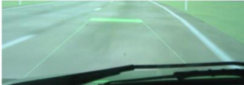
Figure 8: 3D HUD: Drive-path and breaking bar.(adopted from [TON06])
