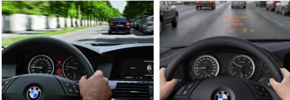
Figure 5: a. (Left)Secondary display used by ACC system. b. (Right) Head-Up Display (courtesy of BMW)
