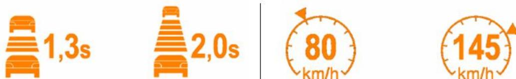
Figure 6: Symbols for desired following distance(left) and wanted speed(right) (adopted from [THO05])
