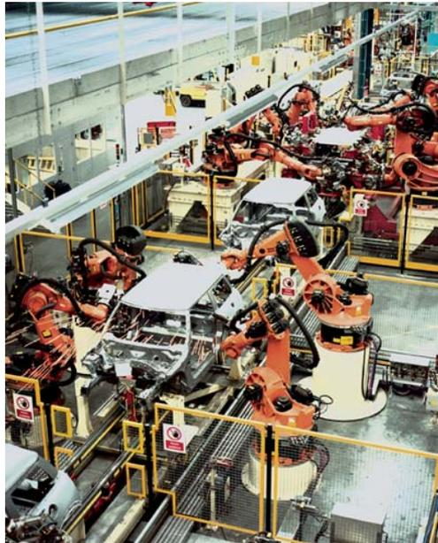
Figure 3.4: welding using robot arms
