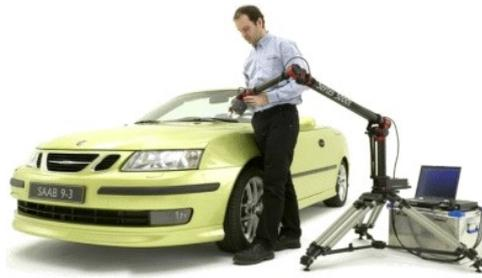
Figure 3.2: semi-automatic scanning of model
