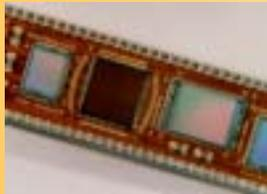
Multichip Module for Radar Evaluation
