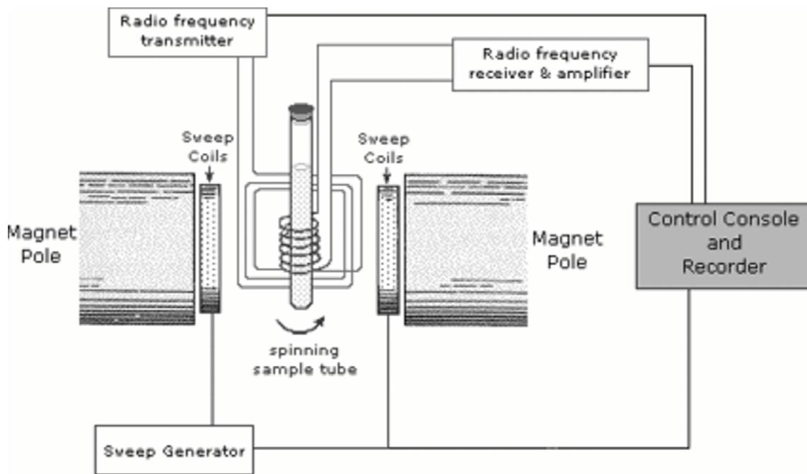
Figure 11: Typical CW NMR spectrometer.
