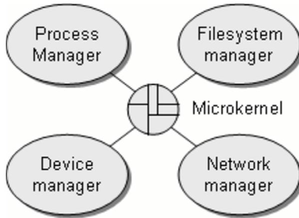
Figure 13: The QNX Microkernel coordinating the system managers.
